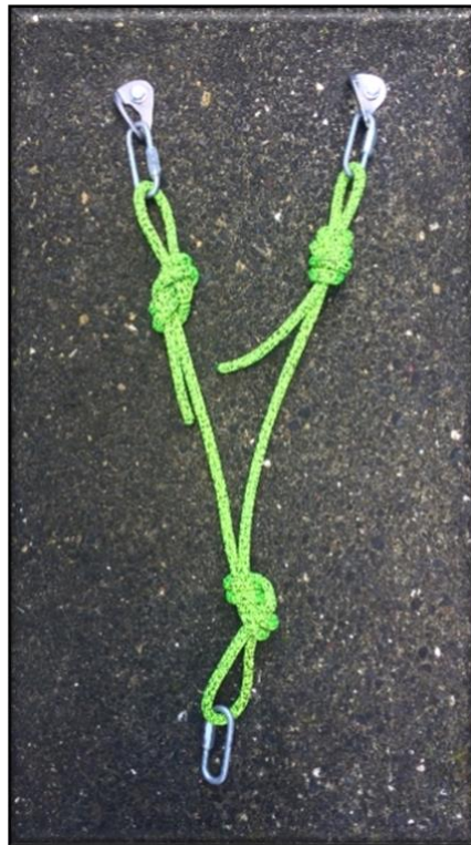
An offcut of 10mm Rope use to create an anchor station.
