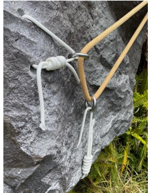
Two threads set up at the start of a safety line. Photo: S Fraser
