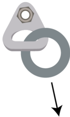
Independent configuration using ring hangers. Arrow indicates direction of load. Picture G Prattley
