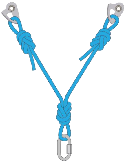
Y Hang configuration using rated 9mm rope Picture: G Prattley
