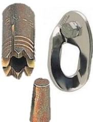
Self-drilling anchors cannot be removed and there is very little margin for error when placing them. However, they *may* be considered acceptable in cases when it was not anticipated that bolts would be needed and a lightweight hand drill kit was carried for use as a last resort.
