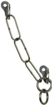
Steel chain that is sold by the meter must be 316 stainless steel or better, must be grade 80 or above, "approved for overhead rigging" and have a rated strength from the manufacturer. Purpose built climbing "belay stations" must meet EN959/UIAA123 standards.
