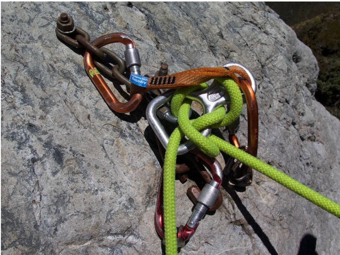
Showing an anchor where the screw link is rusted open.
