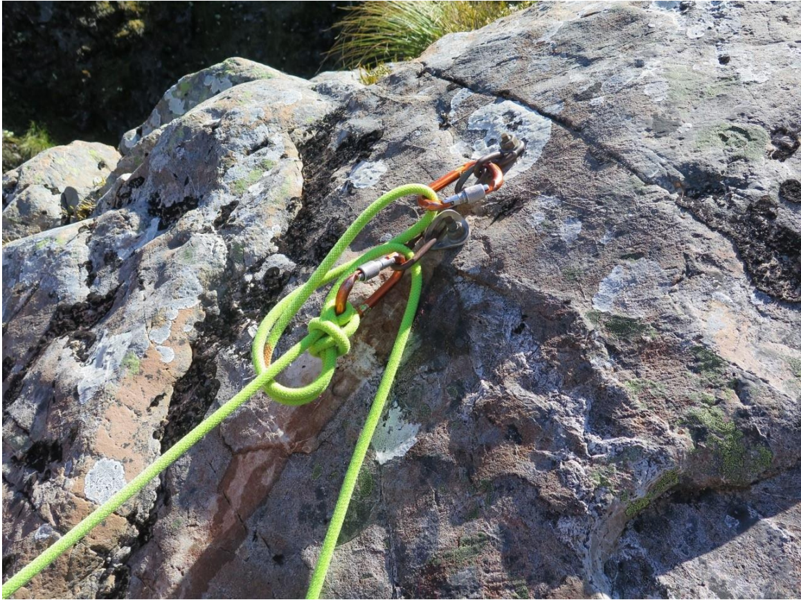
Showing an anchor where the carabiner, although rusted shut, was assessed as OK to use.
